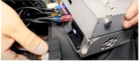
Connect the original plug to the interface socket. Push the black power strip back into the radio.
