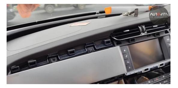
Step 5. Remove the control panel from the display (screws)
