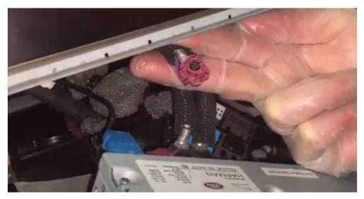
Connect the freed-up video plug to the socket of the other video cable (this can only be done in 1 way).
